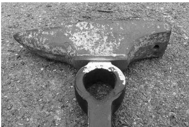
Figure 3: Cavity created by the anvil and vise top. Figure 4 shows the weld between the anvil and the leg. As you can see, they did a fine job filling in the cavities. Next, clean up the welds and grind the sides of the anvil as well as its top so that it aligns with the front jaw.
