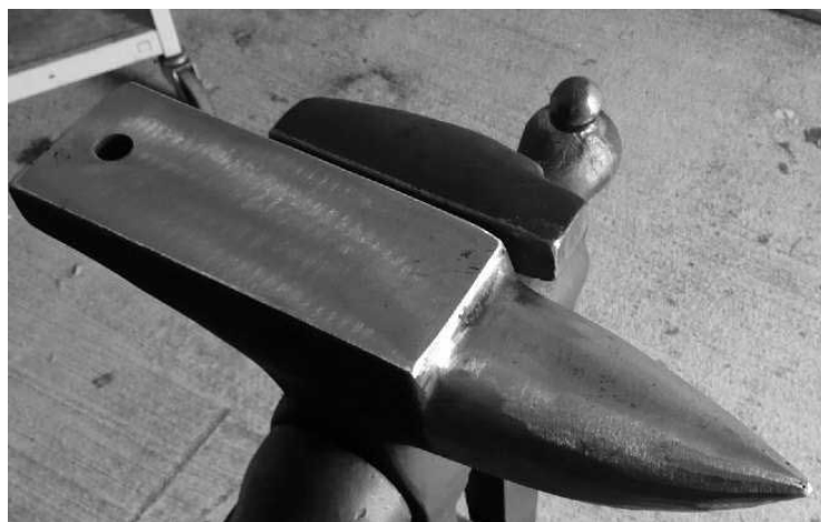
Figure 5: Detail showing jaw overhang. All in all, this was a neat project. I am anticipating years of back-saving use.
