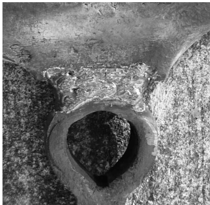
Figure 4: Anvil welded to post.
