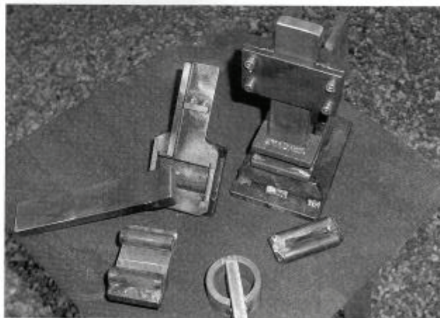
A few of Jim's dies. He often uses this tool under a hydraulic press.
