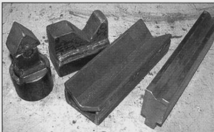
Bending tooling (photo at left). The piece on the right was bought on Ebay. The company selling it sold it by the inch - it's about 6" long.
