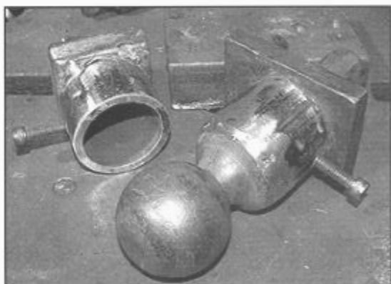
A 2-inch trailer hitch ball welded to a 1 1/2-inch ID pipes makes a handy dishing tool.
