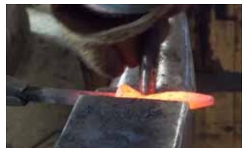
Above two: Punching in the eyes. Note how Bob puts the table of the anvil to good use.
