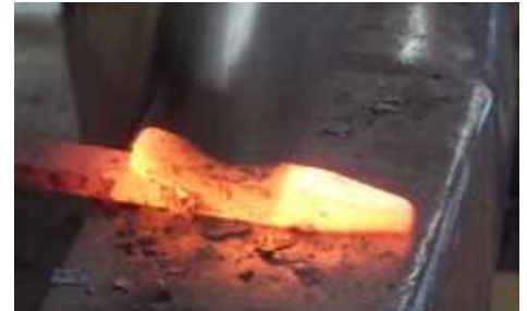
Above: Two shots of the forge welding first step.
