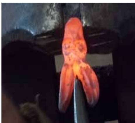
Above: Splitting and spreading out the ears.
