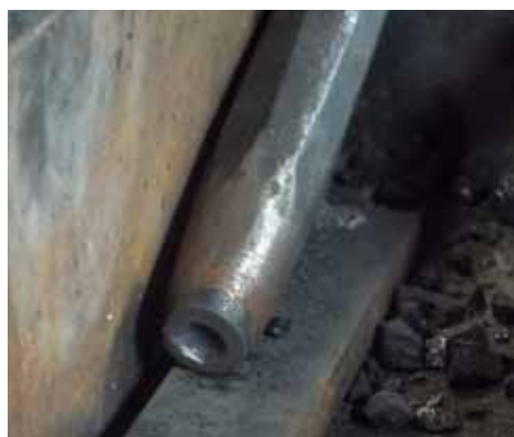
Above: The punch used for the eyes.
