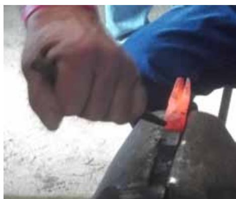
Above: Adding nostrils with a smaller punch.
