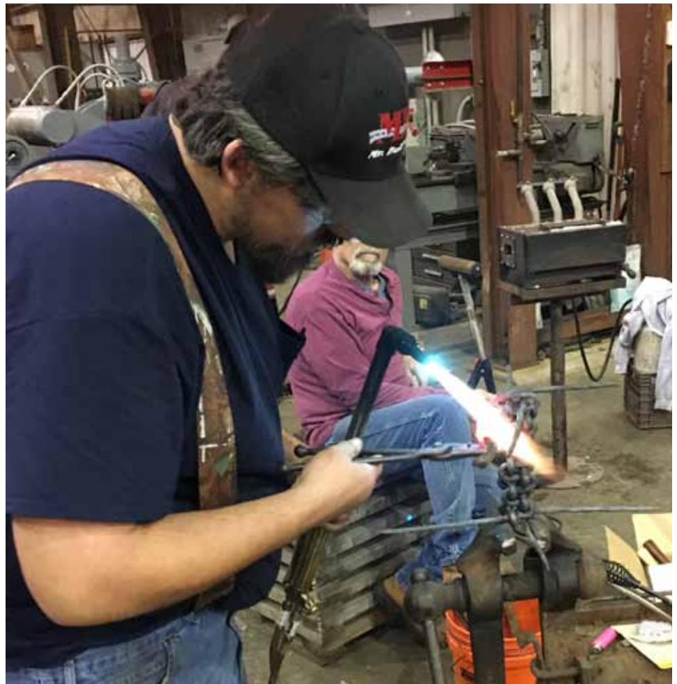
James Hyde demonstrates fabrication of a braided lamp. It is composed of strands of textured round stock, tack welded to start and then torch work to bend and braid. See page 7.
