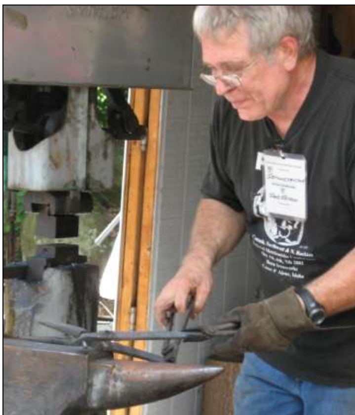
Using a short piece of round stock to make a rivet.
