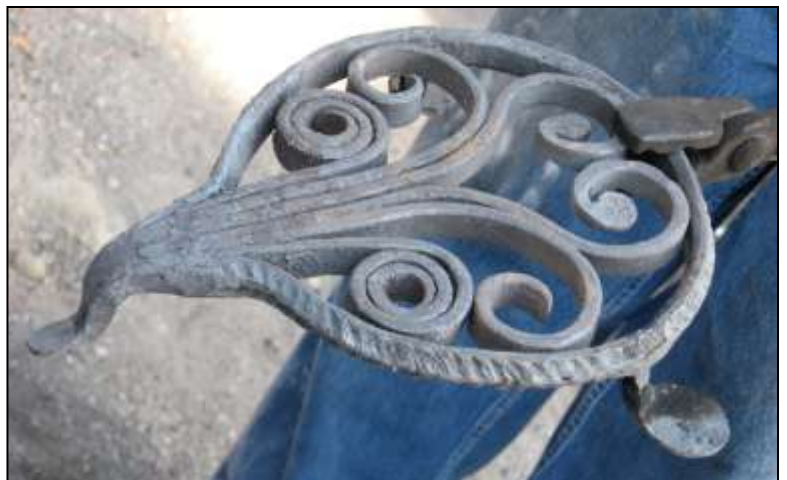
This simple tool has twisted bar welded onto a flat bar with handle. It makes the pattern visible in the picture bellow of the roughly finished trivet Bob Patrick demoed at the Conference
