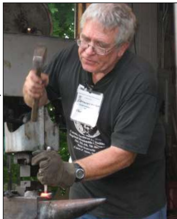
Punching the tongs for a rivet hole
