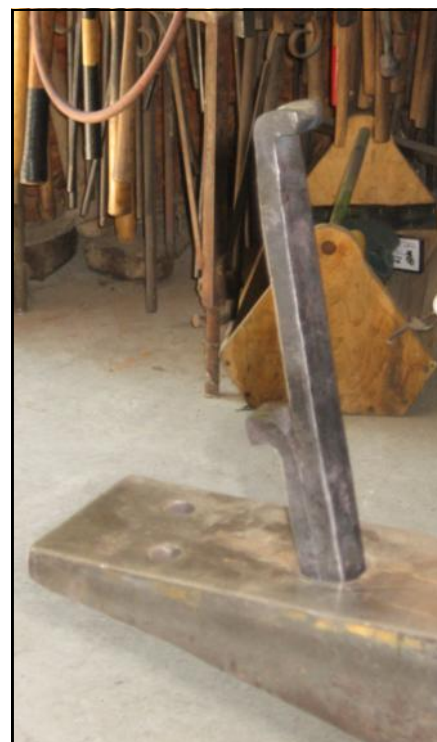
Roy Troutman demonstrating how to make a leaf creaser hardie at the May Hammer-In
