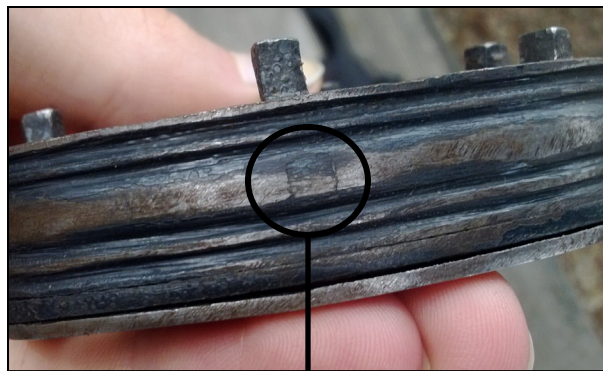
A blind rivet on the side of the same lock shown left. Bill Robertson uses wire for blind rivets that can barely be seen
