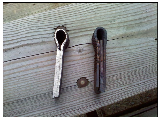
A farrier's rasp is bent into three parts and welded for the tomahawk head (The tang and curved end were cut off first)
