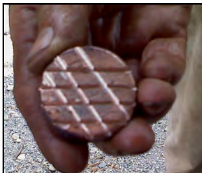
Grind waffled grooves on one face to expose the layers
