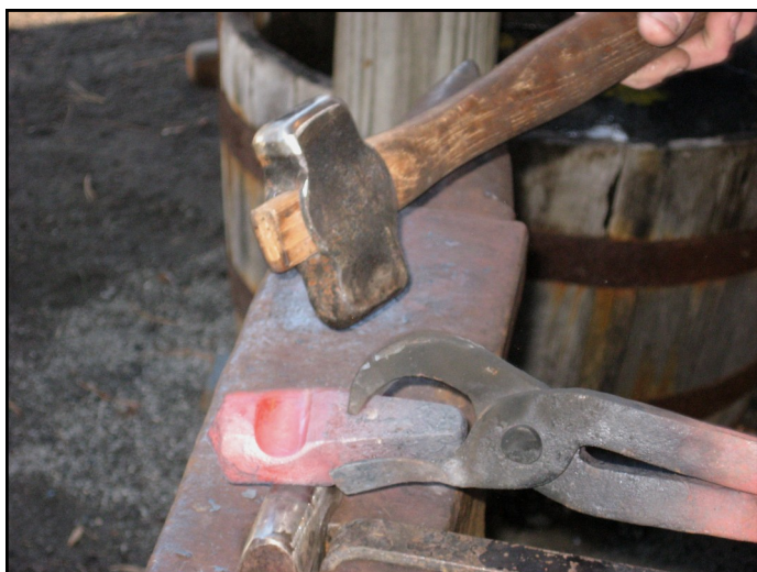
The hardie is fullered into shape
