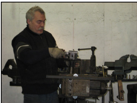
Lathe Vice: adapted to fit into drill press arm
