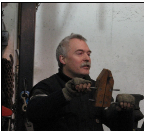
Woodworkers Clamp: good for painted work, odd shapes, and filing in a vice
