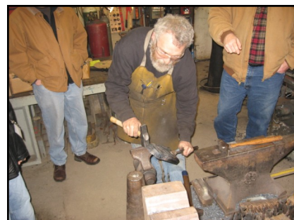
Ken Roby forms the cup of a fireplace shovel on the end of a vice
