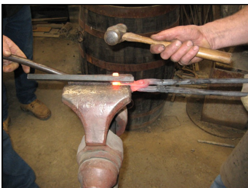
A jig is used to shaped the jaws of the tongs
