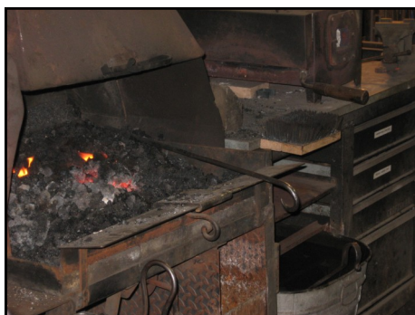
Notice the wire brush that Ken Roby has mounted next to his forge. It is a fast way to brush the iron after every heat
