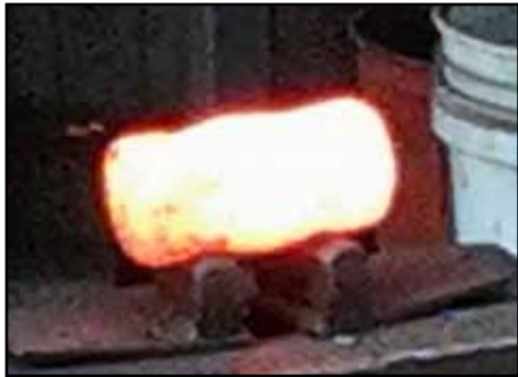
Top: The billet rests in the cup swage waiting for the top swage. Above: A red hot billet rests on the 'monkey swages', which keeps the troughs healthy and supports the piece in a way that prevents any malformation.
