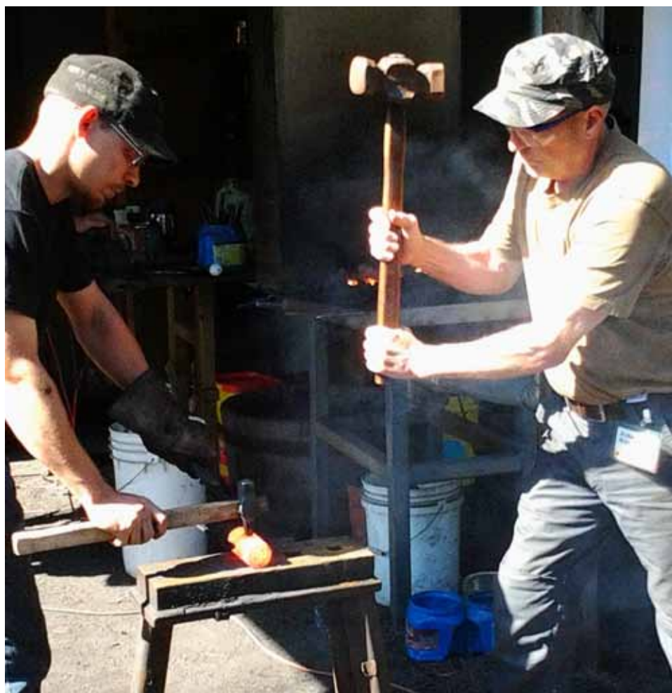
Dave Custer holds the punch and hammer billet as John Klingler supplies the muscle with an 8-pound sledge made by Dave.
