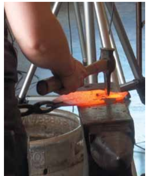
Top: Cutting in details to annealed aluminum (it might be bronze, though). Above: Chamfering the edges of the steel leaf after the deep veins have been cut in.
