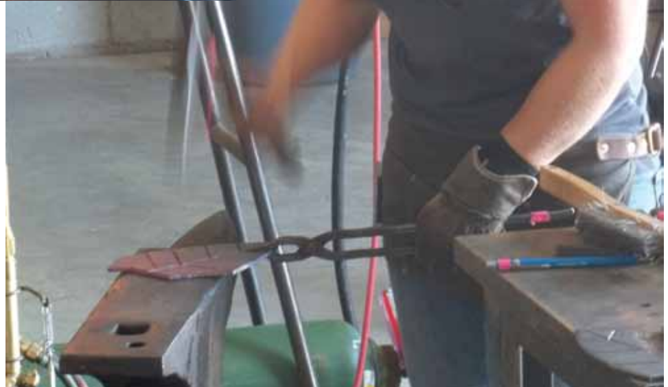
Top: Cutting in details to annealed aluminum (it might be bronze, though). Above: Chamfering the edges of the steel leaf after the deep veins have been cut in.
