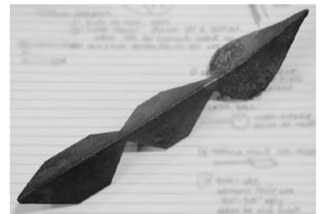
Above: A short length of angle iron nipped to make leaves. The tip has been forged.
